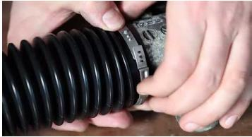
Install the clamp on the steering gearbox end using suitable special pliers.
