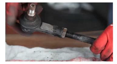
Spray the axial joint with penetrating oil and release the lock nut on the track rod end. Remove the track rod end and clean the thread of the axial joint.
