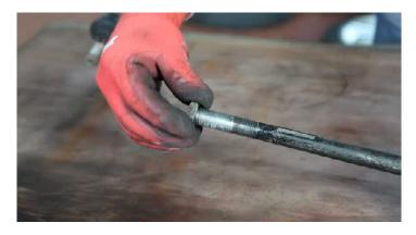
Install the lock nut and the track rod end.
