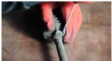
Remove the plastic clamp of the bellows on the side with the track rod end.
