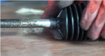
Pull the bellows over the axial joint. The bellows has to engage in the groove of the axial joint. Push the bellows onto the steering gearbox, ensuring that the seal remains in its installed position.
