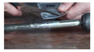
Apply the supplied installation grease to the contact surface of the bellows on the axial joint.
