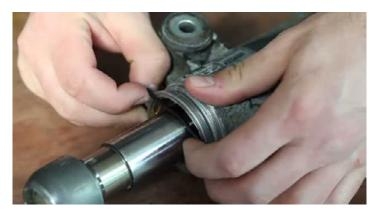
Install the seal from the installation kit on the steering gearbox.
