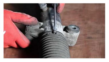
Remove the metal clamp of the bellows on the steering gearbox side.
