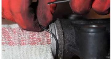
Remove the seal on the steering gearbox.
