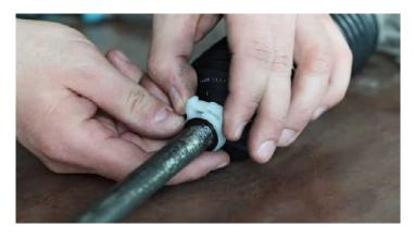
Install the clamp on the axial joint end using suitable special pliers.
