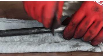
Remove any dirt and traces of corrosion from the contact surface of the bellows on the axial joint. Clean thoroughly with TRW brake cleaner.
