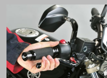
6. Check brake pressure point and free movement of wheel. Clean brake disc.
